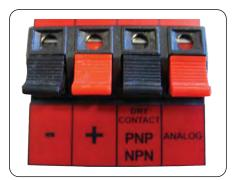
PNP, NPN, 2-wire dry contact and analog sensors can be tested by connecting them suitably to the terminal boards.
